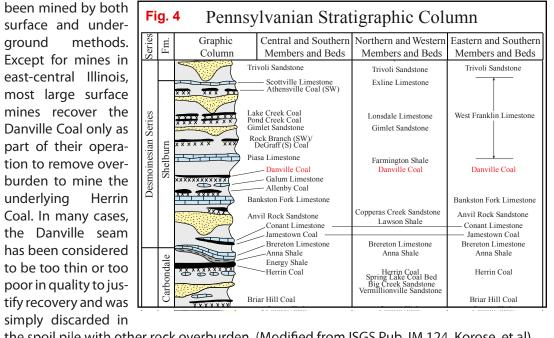
simply discarded in the spoil pile with other rock overburden. (Modified from ISGS Pub. IM 124, Korose, et al)
