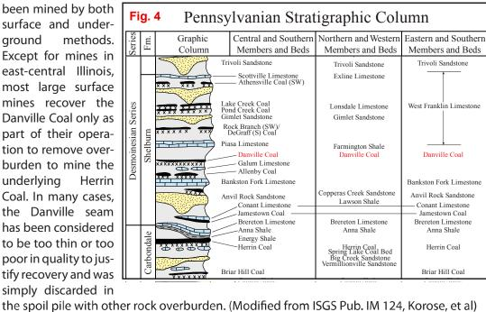
simply discarded in the spoil pile with other rock overburden. (Modified from ISGS Pub. IM 124, Korose, et al)
