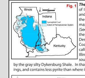
(See Fig 1. and Fig 2.) The Springfield Coal is in the Carbondale formation which is part of the Desmoninesian Series. (See Fig. 4) The Springfield Coal is normally overlain by a black fissile shale called the Turner Mine shale, but in southeastern Illinois, in a belt several miles wide that trends southwestward, the coal is thick and is overlain
