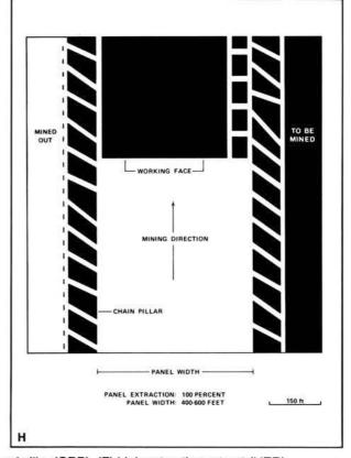
Figure 1 (cont.) Mining methods: (E) checkerboard room and pillar (CRP), (F) high extraction retreat (HER), (G) early (pre-1960) longwall, (H) post-1959 longwall
